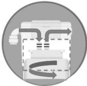
When the Versafilter III is inserted in the filter head and given a ¼ turn, the filter will lock into place and opens the waterway to allow flow into and out of the filter
