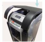
22. Slide your hand over one "finger" at a time near the front to work the snap into place. You will feel and hear it snap when it is properly located. The side may slip to the outside of the side panel. If it does, lift the "finger" and place it closer to the button area.
