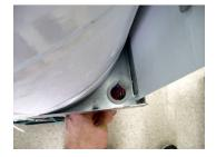
17. Connect wire harness. The 4-pin housings only connect one way.
