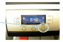
20. After a 2 minute delay, the compressor will run. When snowflake is flashing, lift SS lid slightly to see blue glow.
