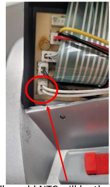
The cold NTC will be the white wire connected to the PCB.
