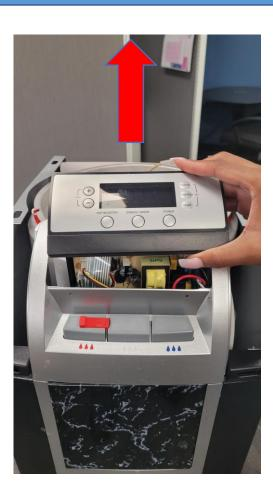
Lift the PCB assembly upward to remove
