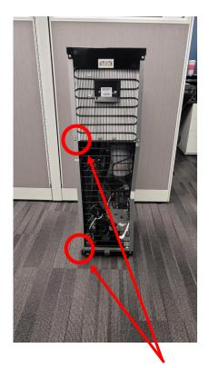
Replace the 2 screws on the back of the side panel
