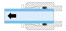
**3.** Push in the collet to release the tubing and then pull the tubing out of the fitting
