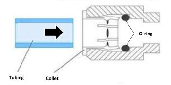
2. Tubing is secured in position. You should be able to pull on the tubing and is will stay locked in place
