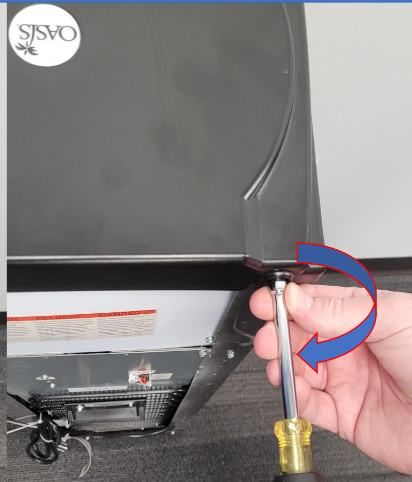
Remove both screws from the cooler top using your 1/4" Nut Driver
